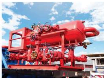
Chock Manifold and Mud Gas Separator
