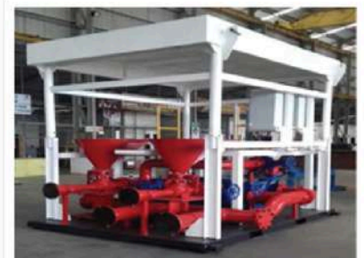
Mud Hopper on Skid
